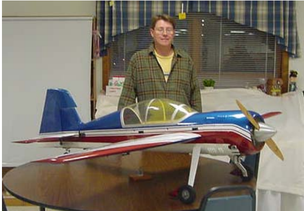
Jim West 25% Great Planes YAK54 81" Wing Span 46cc Brillelli Gas Engine JR 7 Channel Receiver Hitec 645 mg. Servos JR Digital throttle Servo
