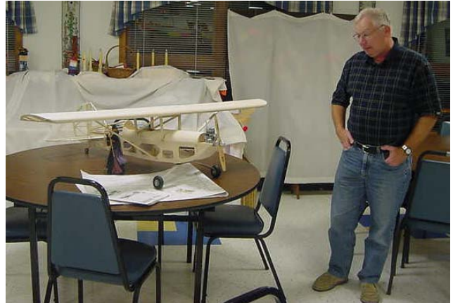
Ron Schippers Great Planes Pete-N-Poke 59.5" Wing Span OS 46 Engine Cream With Light Blue Trim Silk and Dope Finish
