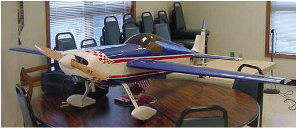
Dan Deirking Hanger 9 Extra 260 Span: 78" Wt. 14.5lbs Power: BME 50 J&A Exhaust
