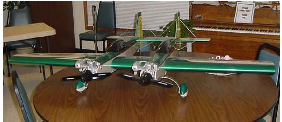
Greg Weseman and his Twin Something Extra. Dual Receiver/Battery 9 Servos Wt. 9 Lbs Wing span: 53" Power two OS 46 AX.
