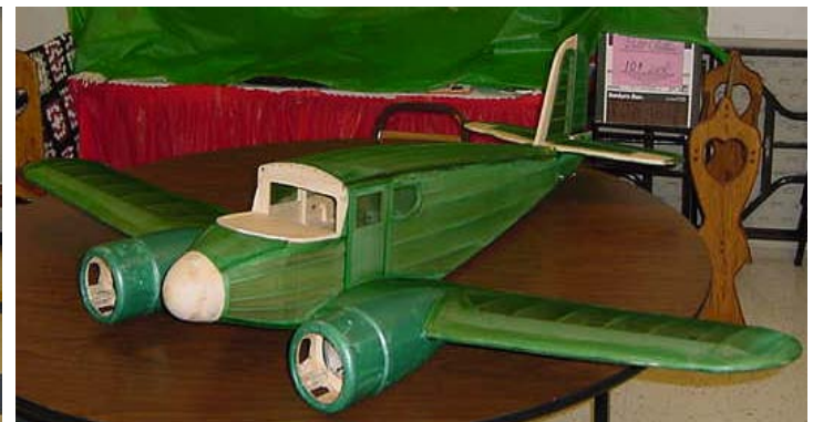
John Rawlings and his UC 78 under Construction. Power: Two OS 25 LA Wingspan 68" Wt. About 3 Lbs. As it sits. Covered with silk and dope.
