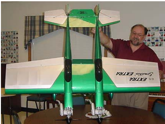
Greg Weseman and his Twin Something Extra. Dual Receiver/Battery 9 Servos Wt. 9 Lbs Wing span: 53" Power two OS 46 AX.
