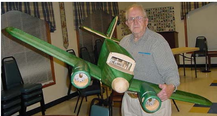
John Rawlings and his UC 78 under Construction. Power: Two OS 25 LA Wingspan 68" Wt. About 3 Lbs. As it sits. Covered with silk and dope.
