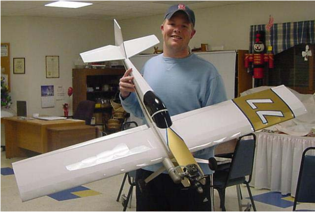
Doug Bruening Sig Four Star 40 Super Tiger 40 Wing Span: 59 3/4" Weight: 4 3/4 Lbs. Never Flown
