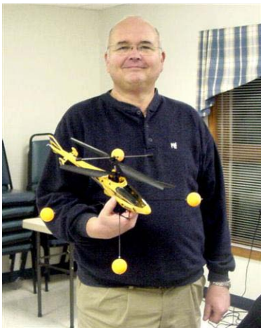
John Bolesta E Flight Blade CX Electric Helicopter Counter rotating blades with dual motors so tail rotor not needed.
