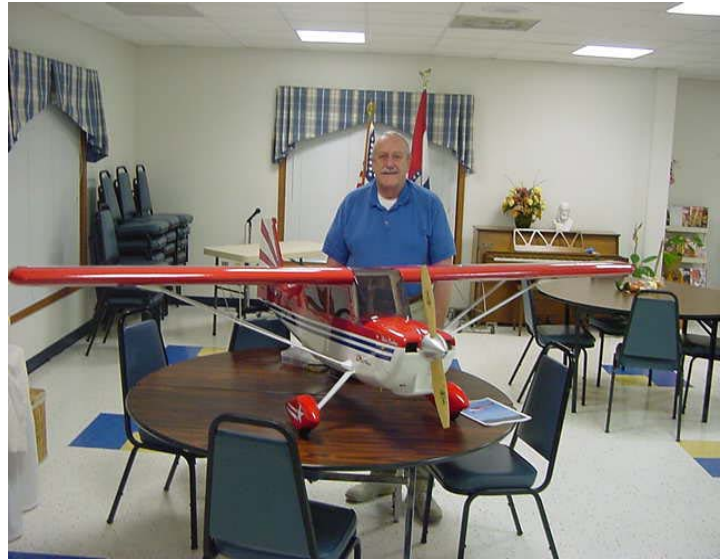
Bob Buss's 25% Super Decathlon Wt. 14 Lbs. Power: SPE 40cc Gas Engine Wingspan 98"
